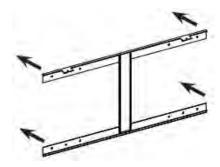
Take away the mounting bracket and then drill four 8mm diameter holes on the wall. Insert the plastic wall plugs into the drilled holes. If installing the appliance on a solid wood wall there is no need to drill the holes in the wood and no need for the plastic wall plug. Fix the mounting bracket using the four screws provided.
