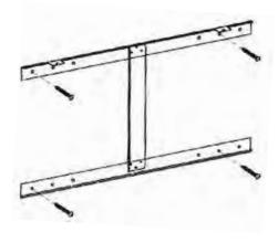
Hang the appliance onto the hooks at the bottom of the bracket and push the top of the appliance into the mounting bracket. Now fix the appliance to the mounting bracket by refitting the two screws which were removed at the beginning.
