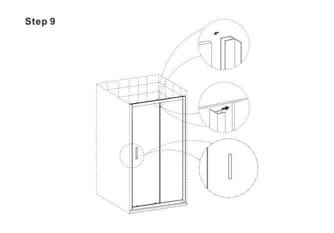
NOTE: WHEN FITTING THE FIXED GLASS PANEL, PLEASE ENSURE A BEAD OF CLEAR SILICONE IS USED ON THE OUTSIDE OF THE GLASS AND REPEAT ON THE OPPOSITE SIDE ONCE THE PANEL IS FIXED IN PLACE.
