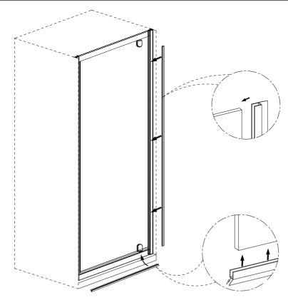
**Note**: when fit the bottom seal, can just be cut as two pieces to fit glass. Or which better
