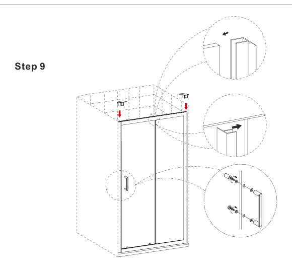
NOTE: WHEN FITTING THE FIXED GLASS PANEL, PLEASE ENSURE A BEAD OF CLEAR SILICONE IS USED ON THE OUTSIDE OF THE GLASS AND REPEAT ON THE OPPOSITE SIDE ONCE THE PANEL IS FIXED IN PLACE.
