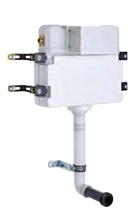
In-Wall Cistern 600(w) x 754(h) x 138-194(d)mm 3/6 Litre flush Ideal for tiled applications All parts serviceable through flush plate aperture 150mm height adjustment Internal isolation valve Top or front flush plate mounting 1/2 BSP, PS insulation jacket
