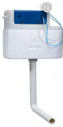
Apex Cistern - Side Inlet 464(w) x 365(h) x 135(d)mm 3/6 Litre flush Side entry inlet valve Top or front flush plate mounting 1/2 BSP, PS insulation jacket, pneumatic flush valve with chrome flush button
