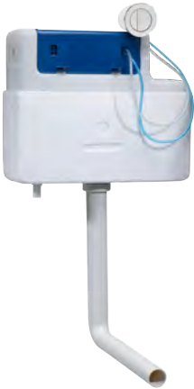
Vortex Cistern - Bottom Inlet 434(w) x 365(h) x 135(d)mm 3/6 Litre flush Bottom entry inlet valve Top or front flush plate mounting 1/2 BSP, PS insulation jacket, pneumatic flush valve with chrome flush button
