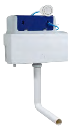
Comfort Height Cistern - Bottom Inlet 437(w) x 324(h) x 165(d)mm 3/6 Litre flush Developed to allow comfort height back to wall pans to be used in 820mm high furniture Bottom entry inlet valve Top or front flush plate mounting 1/2 BSP, PS insulation jacket, pneumatic flush valve with chrome flush button
