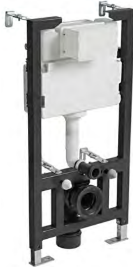
1000mm Wall Hung WC Frame with Front Operated Cistern 500(w) x 1000(h) x 167-215(d)mm 3/6 Litre flush Ideal for boxed-in applications Requires flush plate/button or contactless sensor 200mm height adjustment
